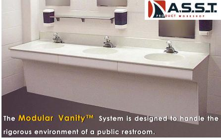
Created by ASST, this innovative wall hung vanity system utilizes a sturdy aluminum and polyethylene support structure with a thermoformed 1/4" thick removable (solid surface or resin) front panel allowing for easy access to plumbing. The vanity system is available in 30" wide increments and includes both a backsplash, side panels and a **DuPont Corian®** #810 integral sink bowl.
